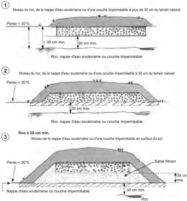
**Figure B.15.3 : La fosse de rétention construite sur place**
